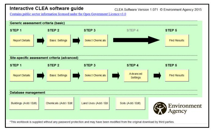
**Box 1**: CLEA model process flow diagram indicating the key steps in deriving Generic Assessment Criteria (GAC) or Site Specific Assessment Criteria (SSAC) [source: UK Environment Agency]
